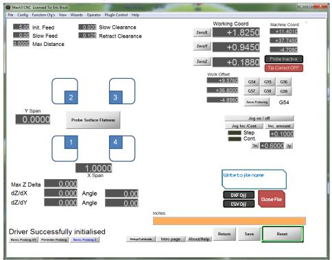
The Basic Z Surface page is only meant to provide a very basic check of how flat the surface of your object is relative to the X-Y plane of the machine. You can probe in the X only, Y only, or an X-Y square pattern to determine if your part is 'level' and or of a constant thickness. It is useful to determine if your part is bowed or tipped in your fixturing for operations that require a very flat and level surface, such as engraving.
