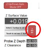
This LED is used as a 'safety' and must be turned on by first probing an initial surface using the 'Initial Z Surface to set Z' button before the auto up/down routines will function. This is used to ensure that the surface and probing depths are 'known' so safety checks can be used to prevent crashing the probe.
