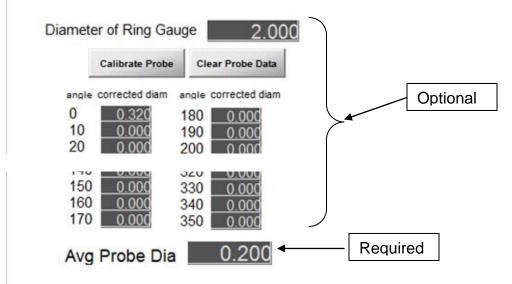
NOTE: You are not required to run the calibration routine to do any of the probing routines, but you must have a value entered in to the 'Avg Probe Dia' DRO to be used as a default.
