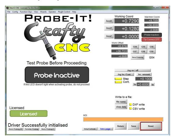
I would also recommend that as you learn how to probe with the software you are using, that you start by test probing into loosely clamped items or your finger to ensure it behaves as you think it will.
